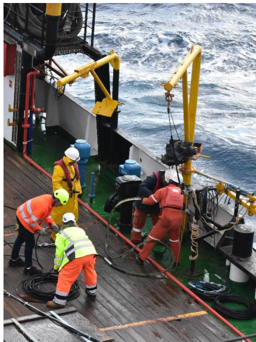
Photo 34: Installing hydrophone for Passive Acoustic Monitoring (PAM)
