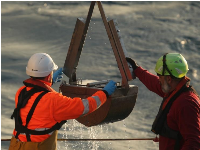
Photo 25: Sediment sampling with stainless-steel ETS_85A Van Veen grab
