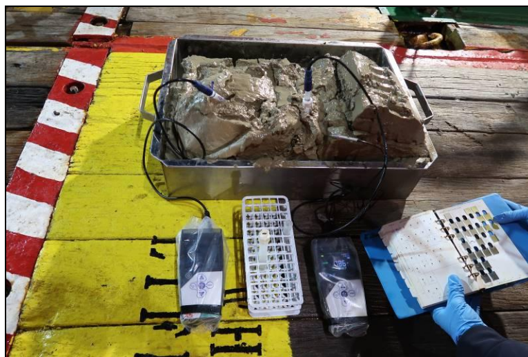
Figure 10 – Measurement of physico-chemical properties of sediments and comparing the colour of sediment with a Munsell soil colour charts
