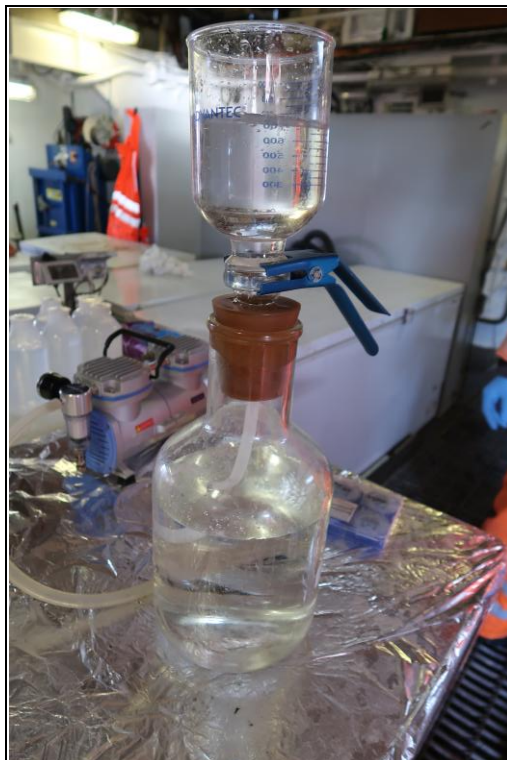
Figure 7 –Pressure pump for water filtration
