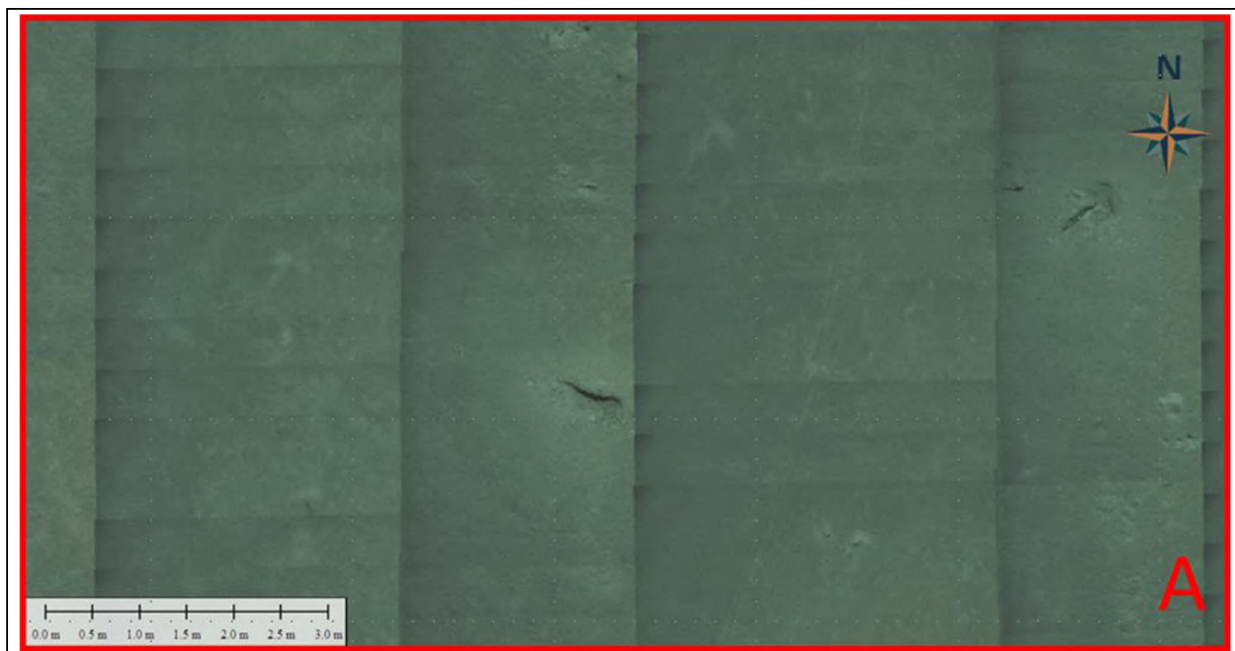
Figure 54 - Detailed view of traces left by Van Veen grab sampler at D3b location
