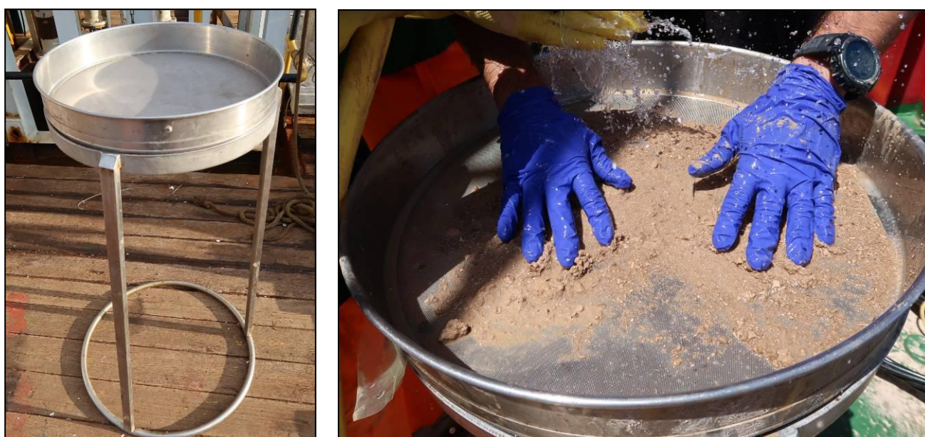
Figure 11 – Benthos Sieve set-up prior to operations (left) and during Sample Washing and Processing (right)
