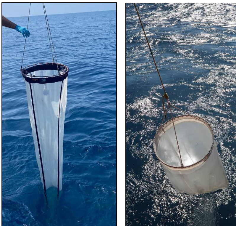
Figure 8 – Zooplankton (left) and Ichthyoplankton Sampling (right) Using WP2 net
