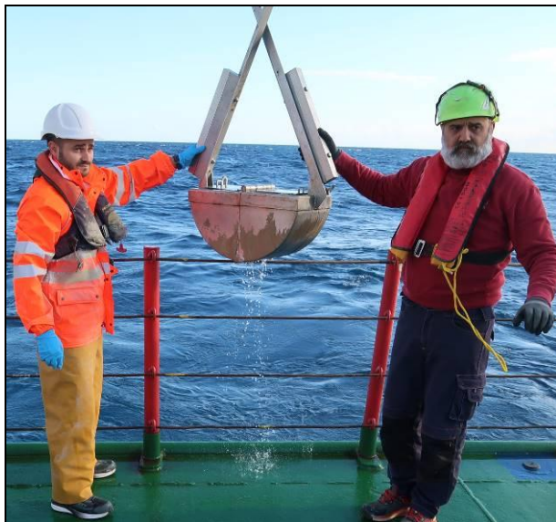
Figure 9 – Van Veen Grab Deployment (left) and Sample Description prior to Sub-Sampling (right)
