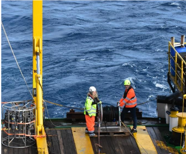
Figure 14-30: Installing hydrophone for PAM
