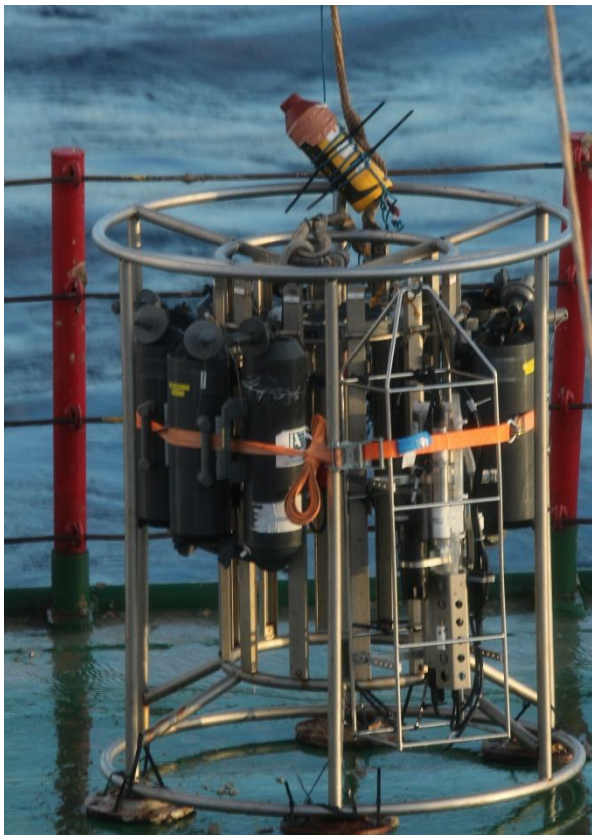
Figure 14-24: Water quality sampling with General Oceanics Model 1018 (MWS12) Rosette multisampler
