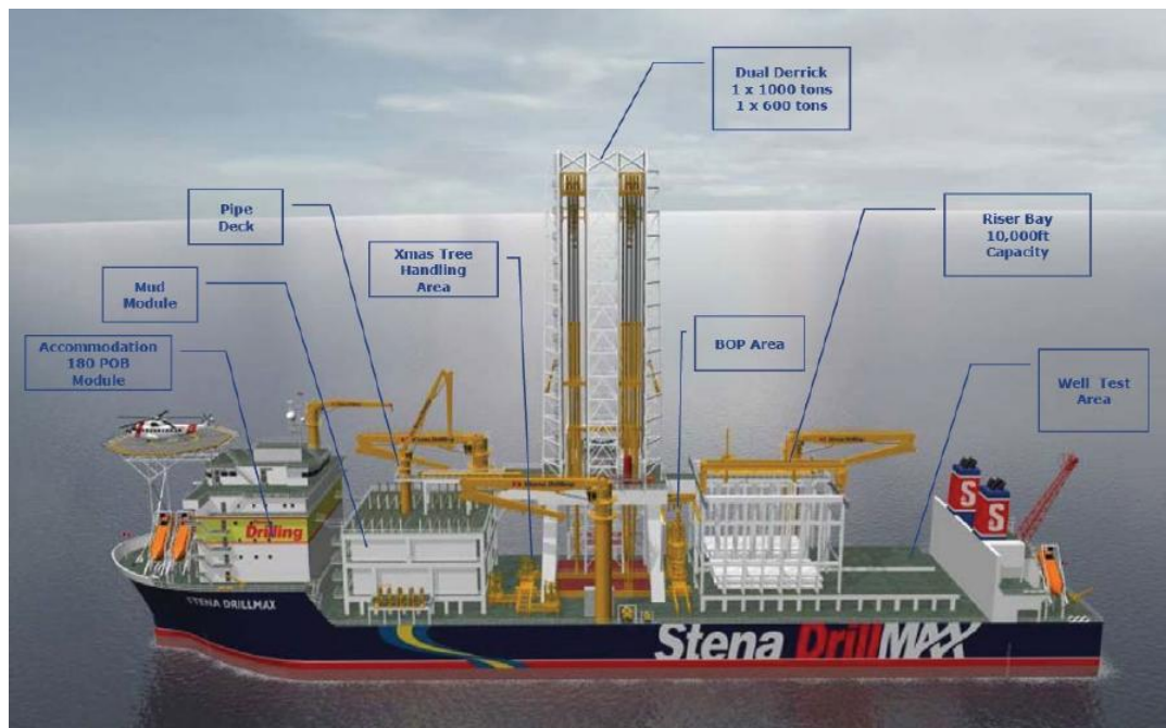
Figure 9-3: MODU Facility Layout
