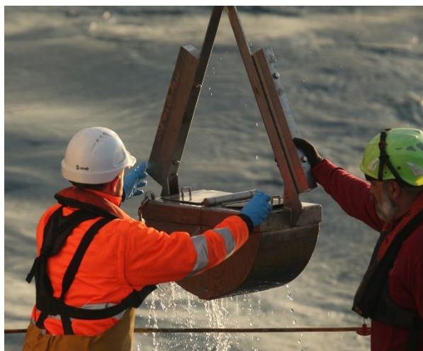
Figure 14-20: Sediment sampling with stainless-steel ETS_85A Van Veen grab
