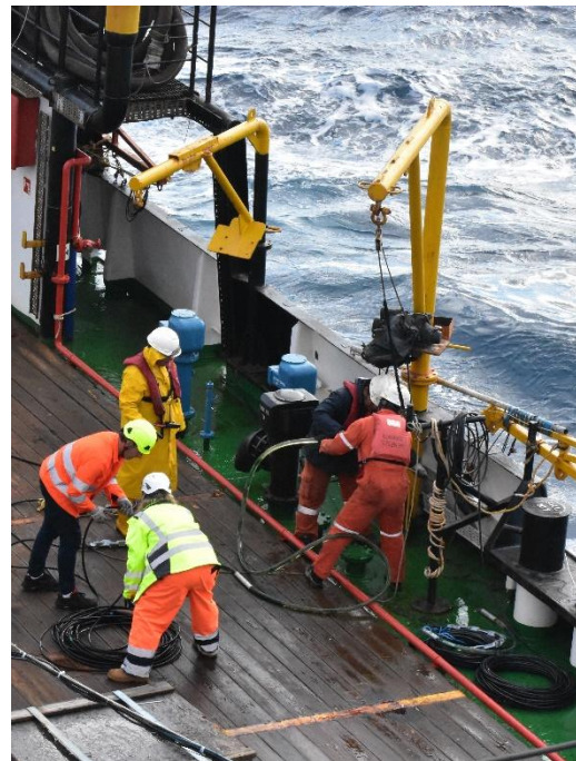
Figure 14-29: Installing hydrophone for Passive Acoustic Monitoring (PAM)
